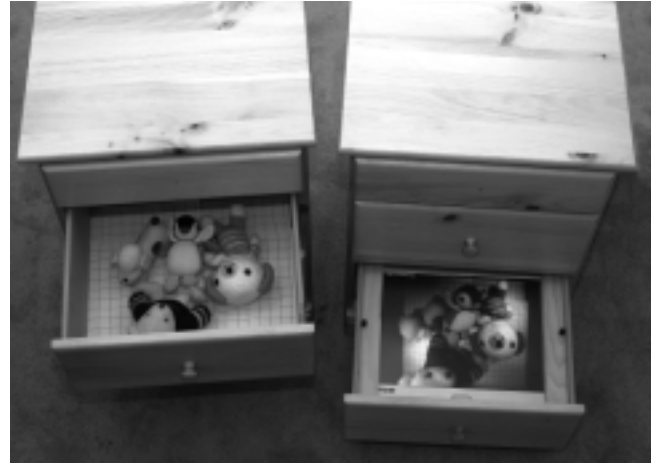
Figure 1. A prototype of a pair of Peek-A-Drawers. The contents of the upper drawer (left) are displayed in the lower drawer of the other chest (right).
